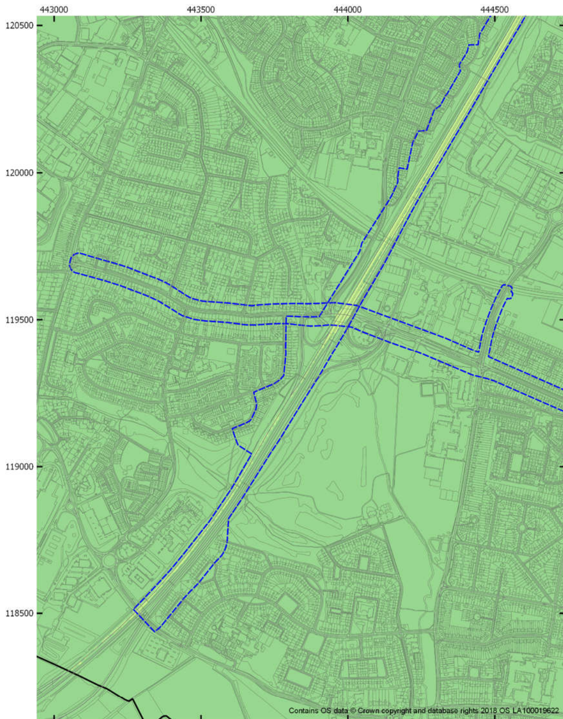
Figure 5-23 Short term NO 2 concentration model results for 2036 SGO D1 scenario AQMA No. 1 (A335 / Eastleigh) (West)
