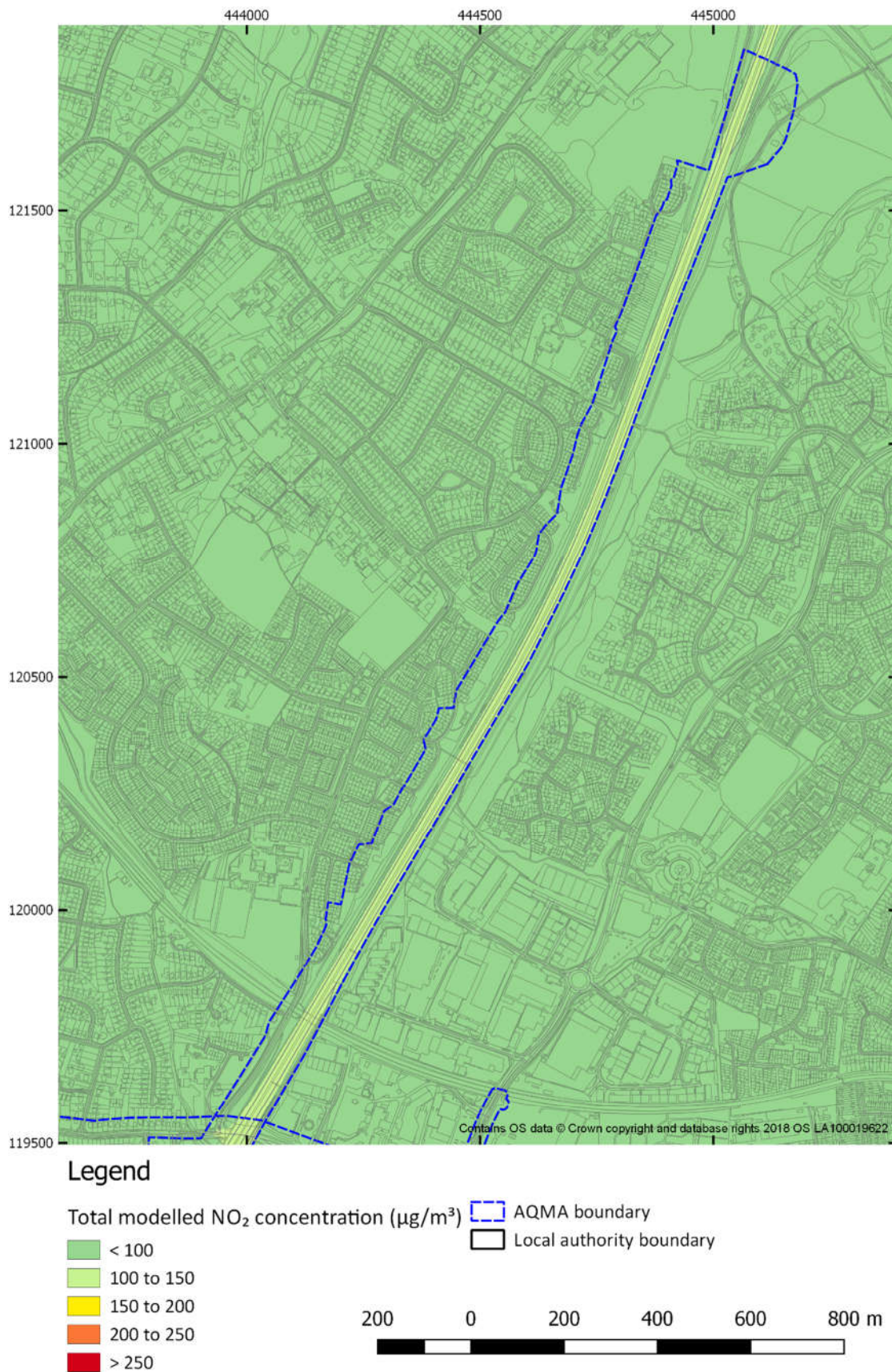
Figure 5-27 Short term NO 2 concentration model results for pseudo-2030 SGO C scenario AQMA No. 2 (M3) (North)
