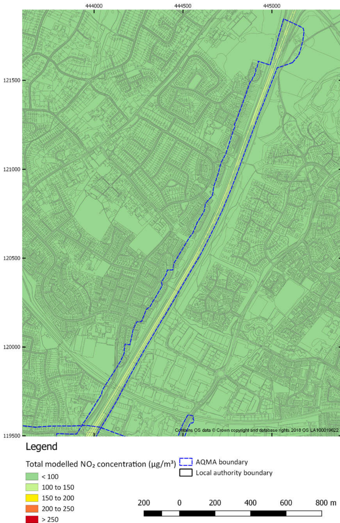
Figure 5-31 Short term NO 2 concentration model results for 2036 SGO C scenario AQMA No. 2 (M3) (North)
