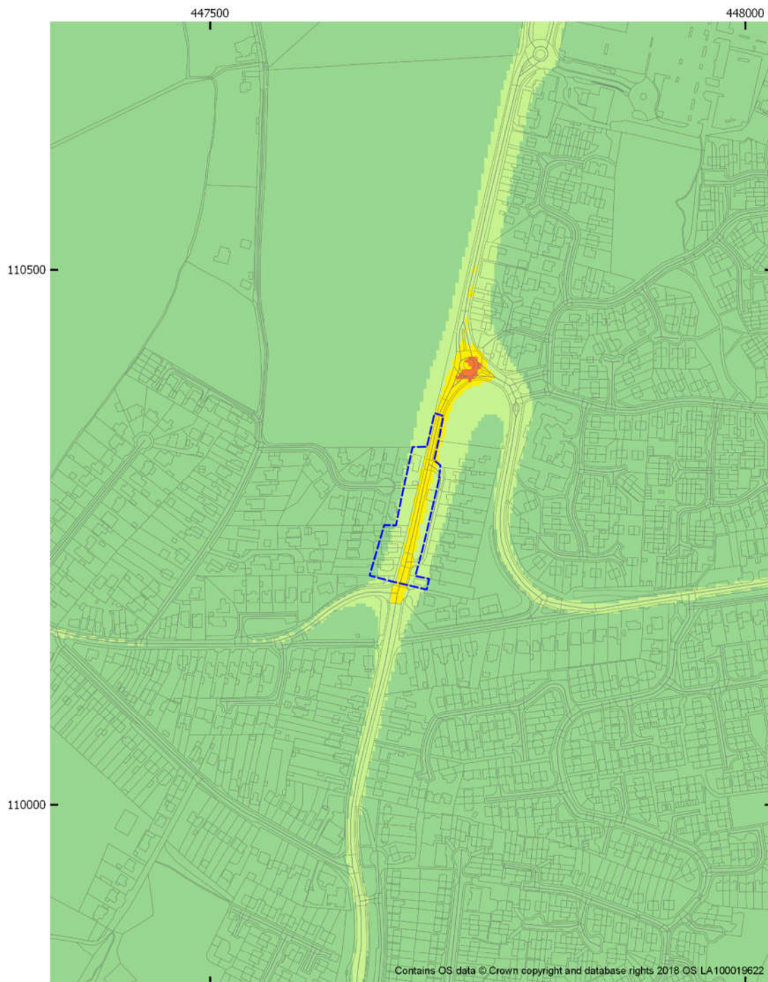
Figure 6-39 Short term PM 10 concentration model results for pseudo-2030 SGO E scenario AQMA No. 3 (Hamble Lane)
