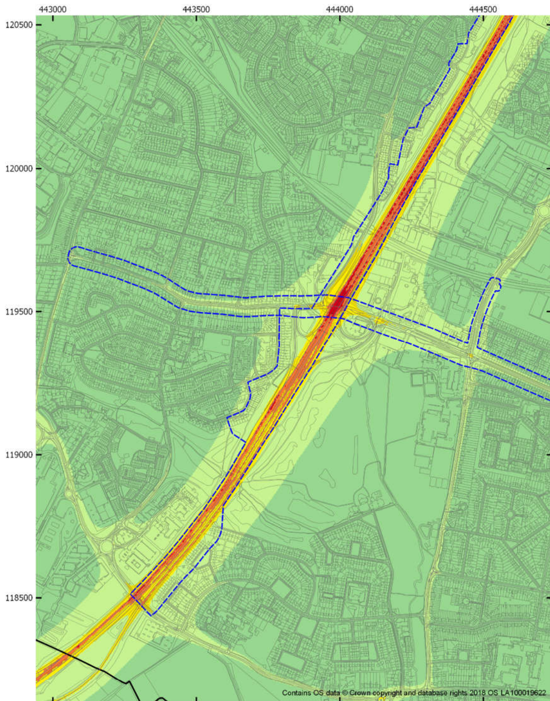
Figure 3-22 Annual mean PM 10 concentration model results for 2036 SGO C scenario AQMA No. 1 (A335 / Eastleigh) (West)
