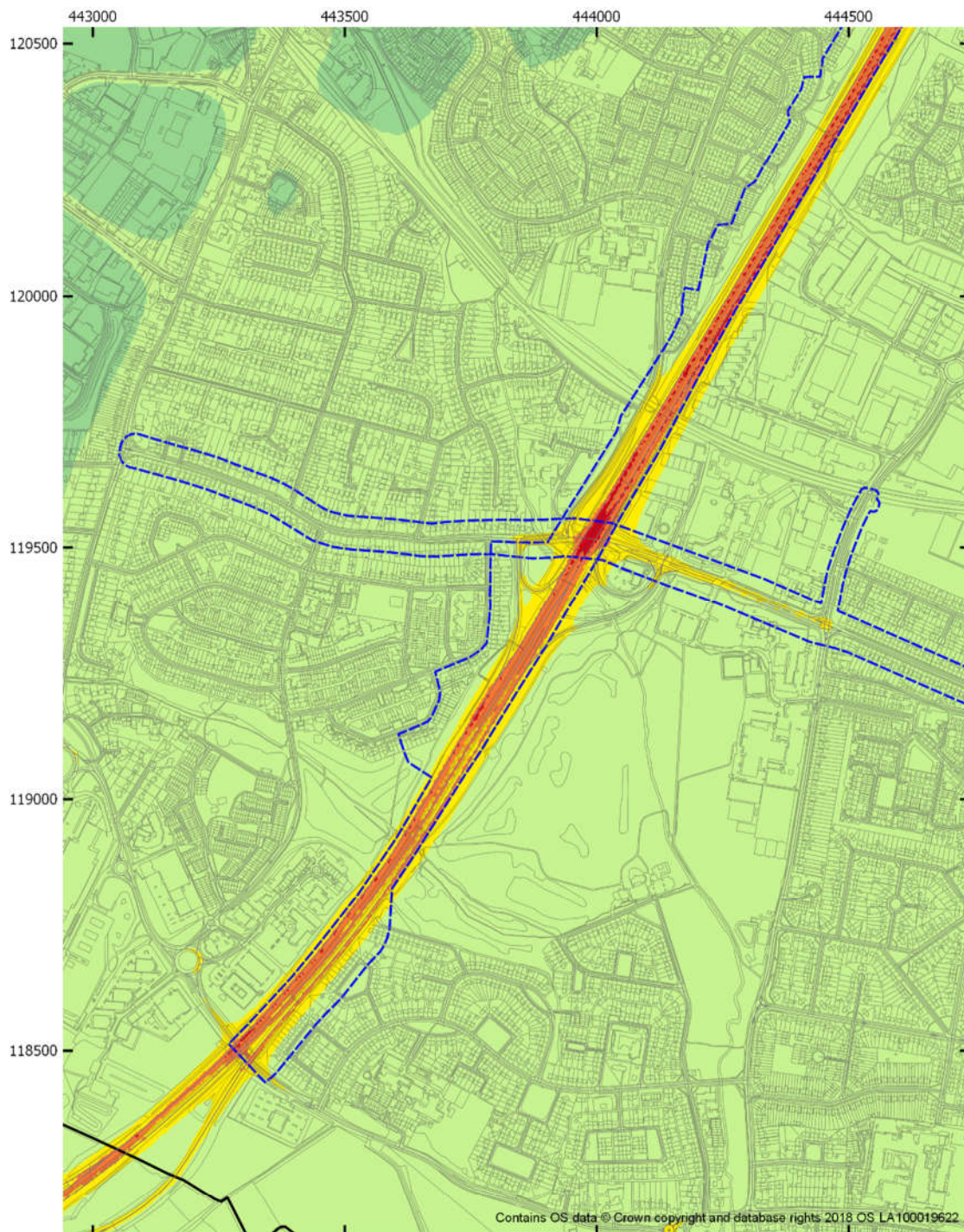
Figure 4-22 Annual mean PM 2.5 concentration model results for 2036 SGO C scenario AQMA No. 1 (A335 / Eastleigh) (West)
