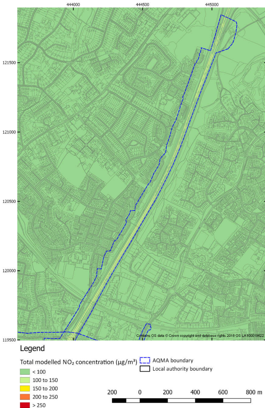
Figure 5-35 Short term NO 2 concentration model results for 2036 Baseline AQMA No. 2 (M3) (North)
