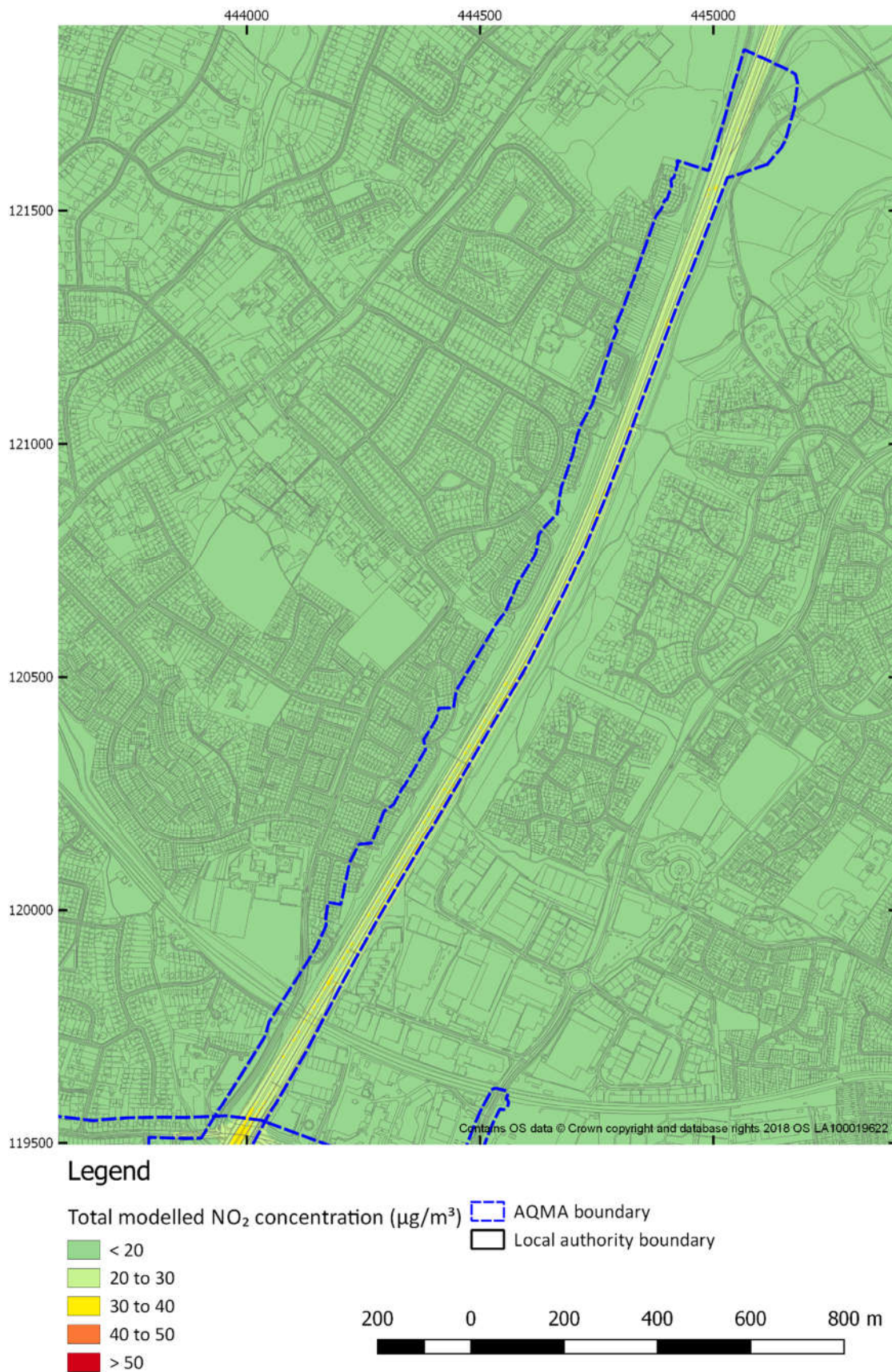
Figure 2-34 Annual mean NO 2 concentration model results for 2036 SGO E scenario AQMA No. 2 (M3) (North)
