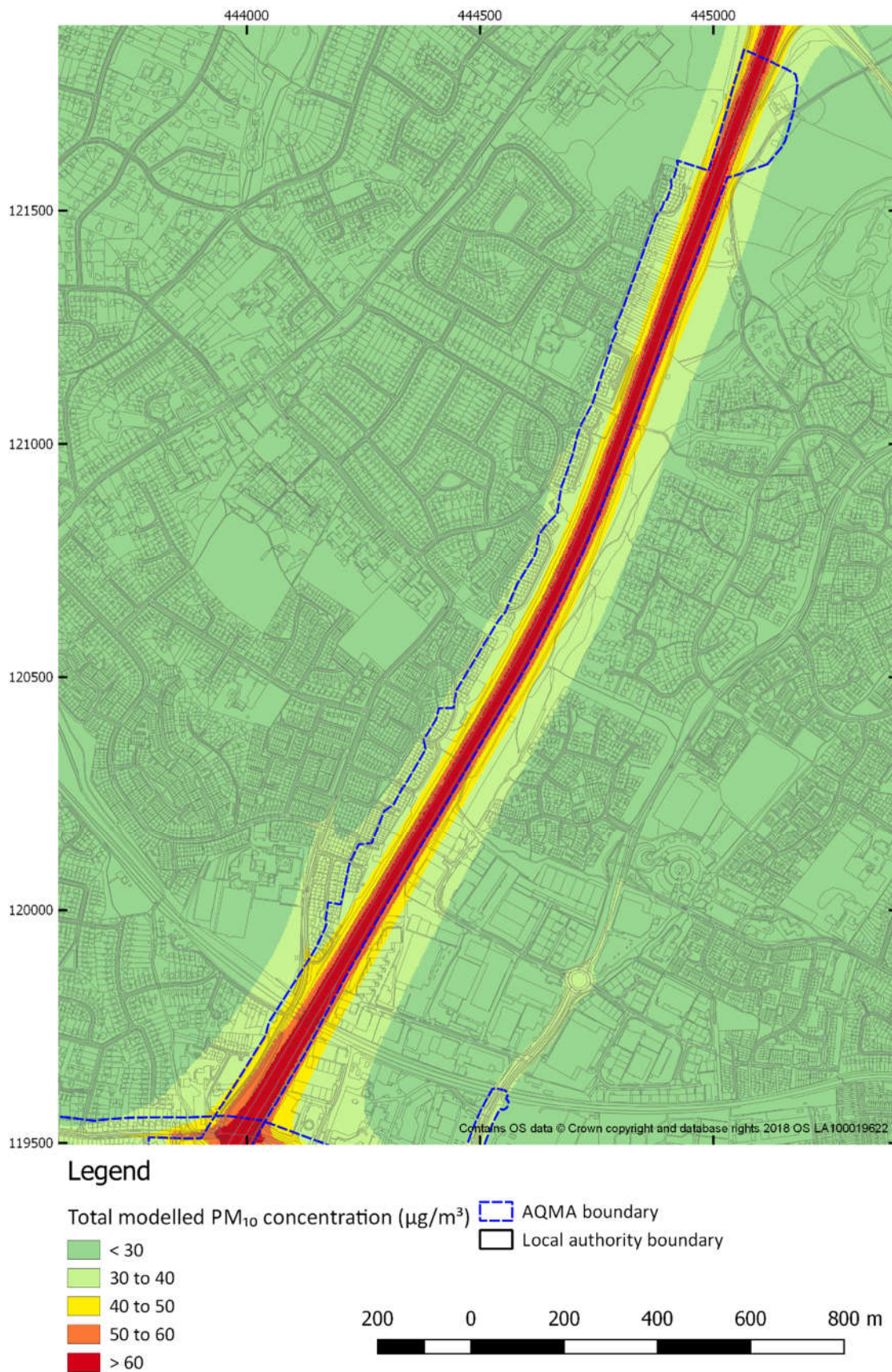
Figure 6-35 Short term PM 10 concentration model results for 2036 Baseline AQMA No. 2 (M3) (North)
