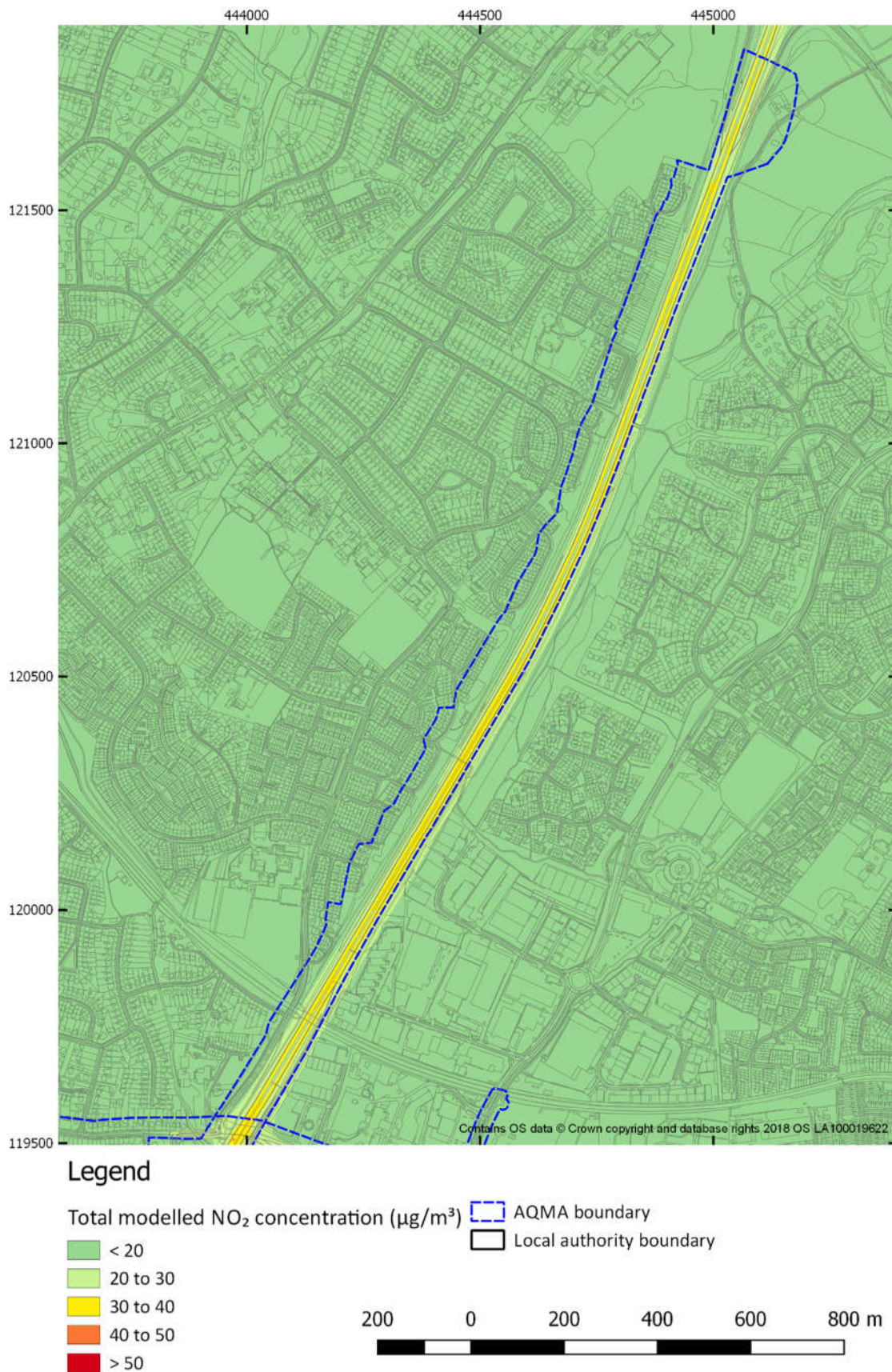
Figure 2-28 Annual mean NO 2 concentration model results for pseudo-2030 SGO D1 scenario AQMA No. 2 (M3) (North)
