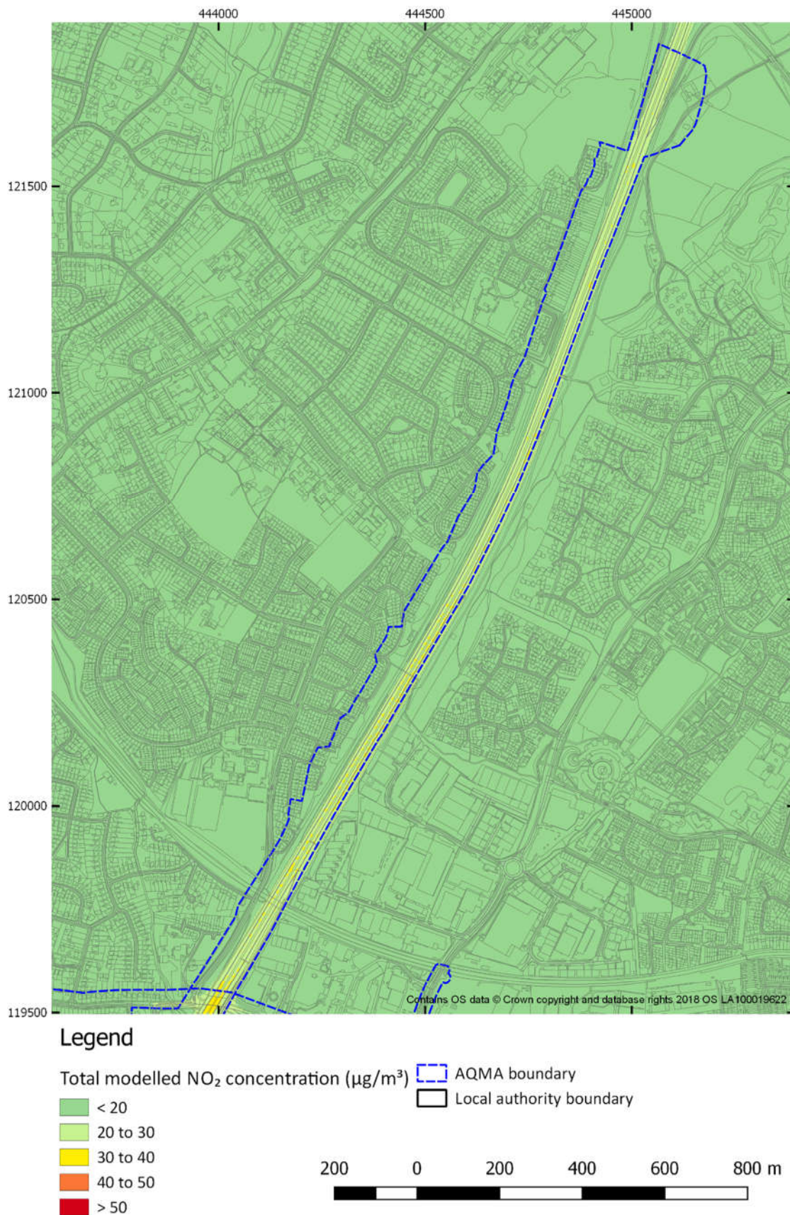
Figure 2-31 Annual mean NO 2 concentration model results for 2036 SGO C scenario AQMA No. 2 (M3) (North)
