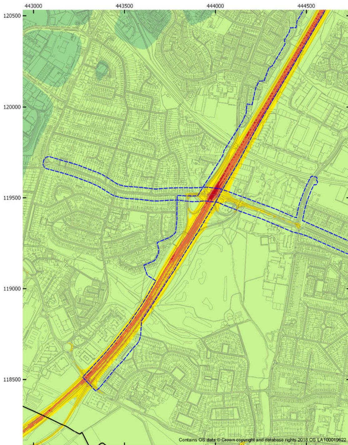
Figure 4-24 Annual mean PM 2.5 concentration model results for 2036 SGO D2 scenario AQMA No. 1 (A335 / Eastleigh) (West)
