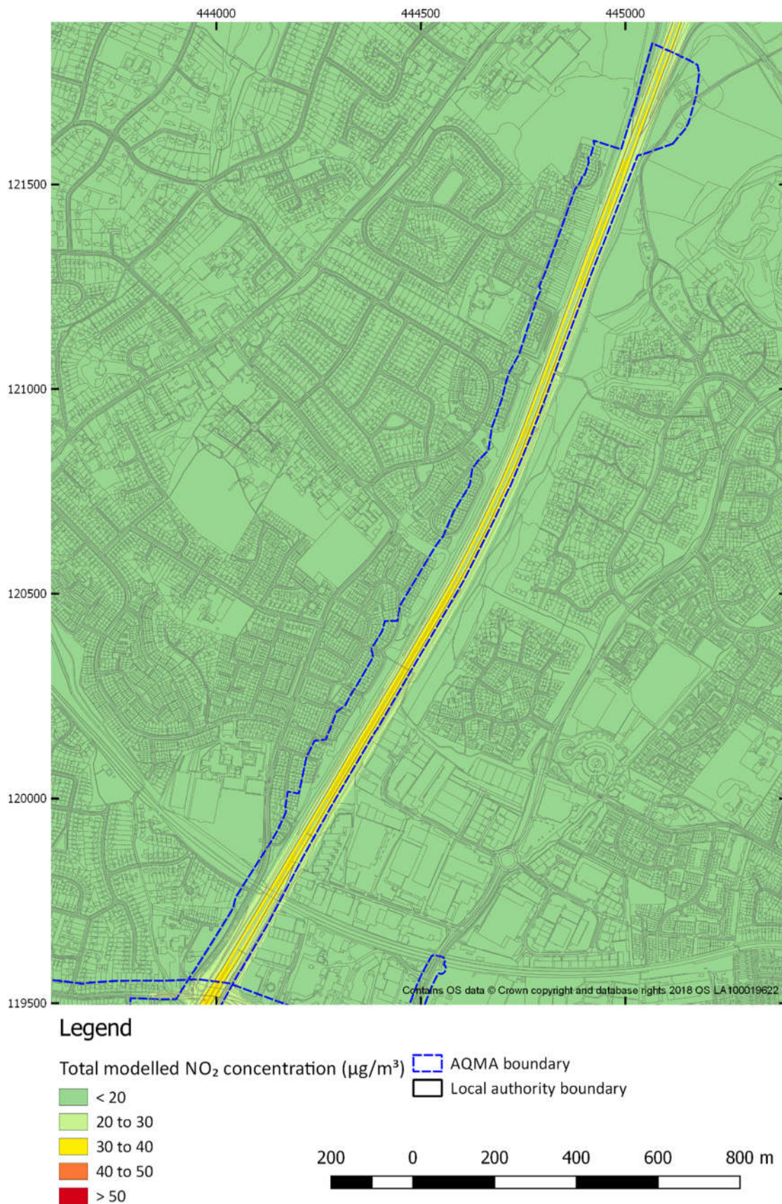
Figure 2-27 Annual mean NO 2 concentration model results for pseudo-2030 SGO C scenario AQMA No. 2 (M3) (North)
