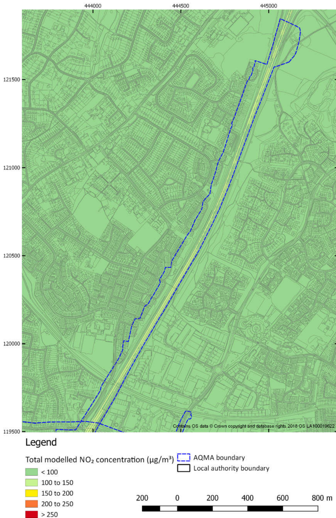
Figure 5-33 Short term NO 2 concentration model results for 2036 SGO D2 scenario AQMA No. 2 (M3) (North)
