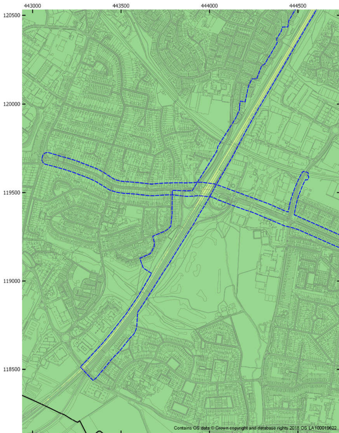
Figure 5-25 Short term NO 2 concentration model results for 2036 SGO E scenario AQMA No. 1 (A335 / Eastleigh) (West)
