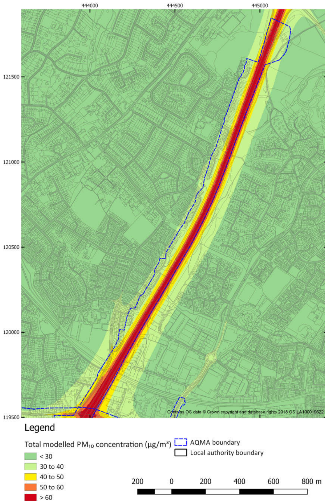
Figure 6-28 Short term PM 10 concentration model results for pseudo-2030 SGO D1 scenario AQMA No. 2 (M3) (North)
