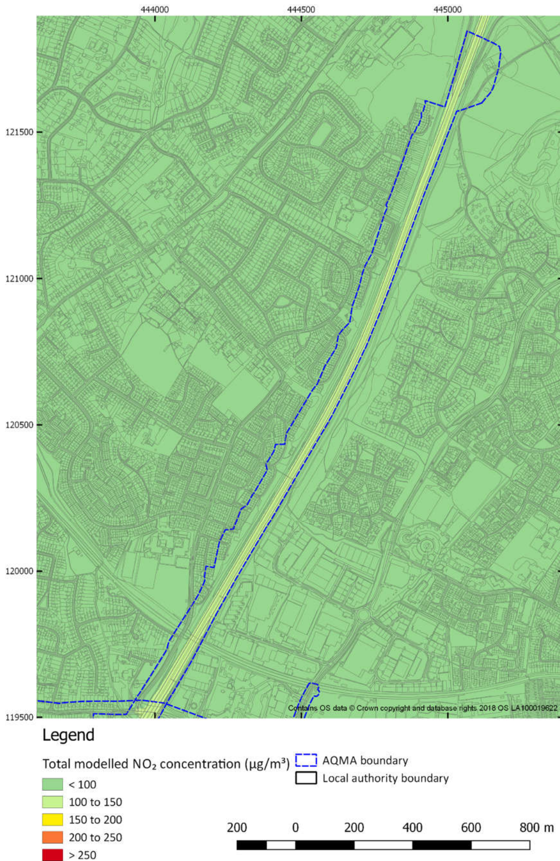
Figure 5-29 Short term NO 2 concentration model results for pseudo-2030 SGO D2 scenario AQMA No. 2 (M3) (North)
