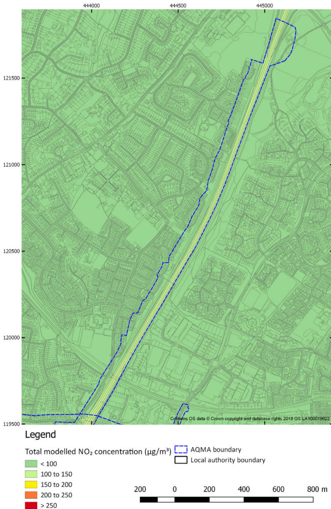
Figure 5-30 Short term NO 2 concentration model results for pseudo-2030 SGO E scenario AQMA No. 2 (M3) (North)
