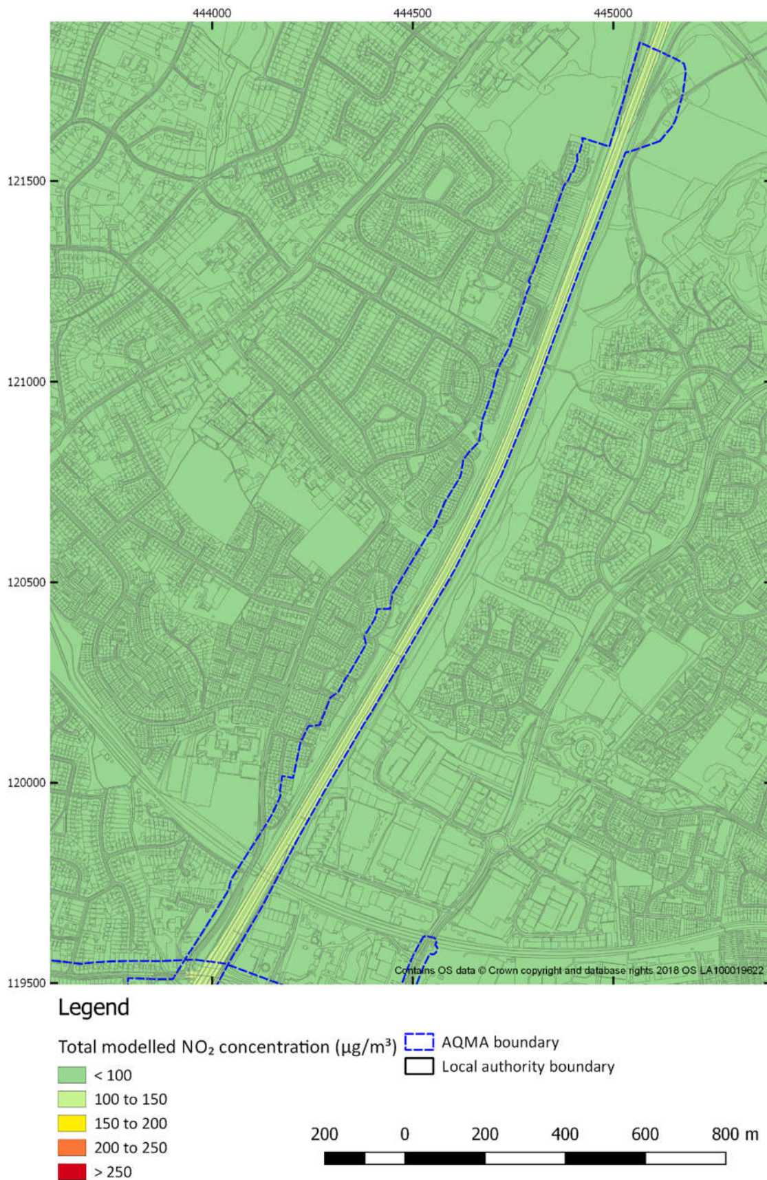
Figure 5-28 Short term NO 2 concentration model results for pseudo-2030 SGO D1 scenario AQMA No. 2 (M3) (North)
