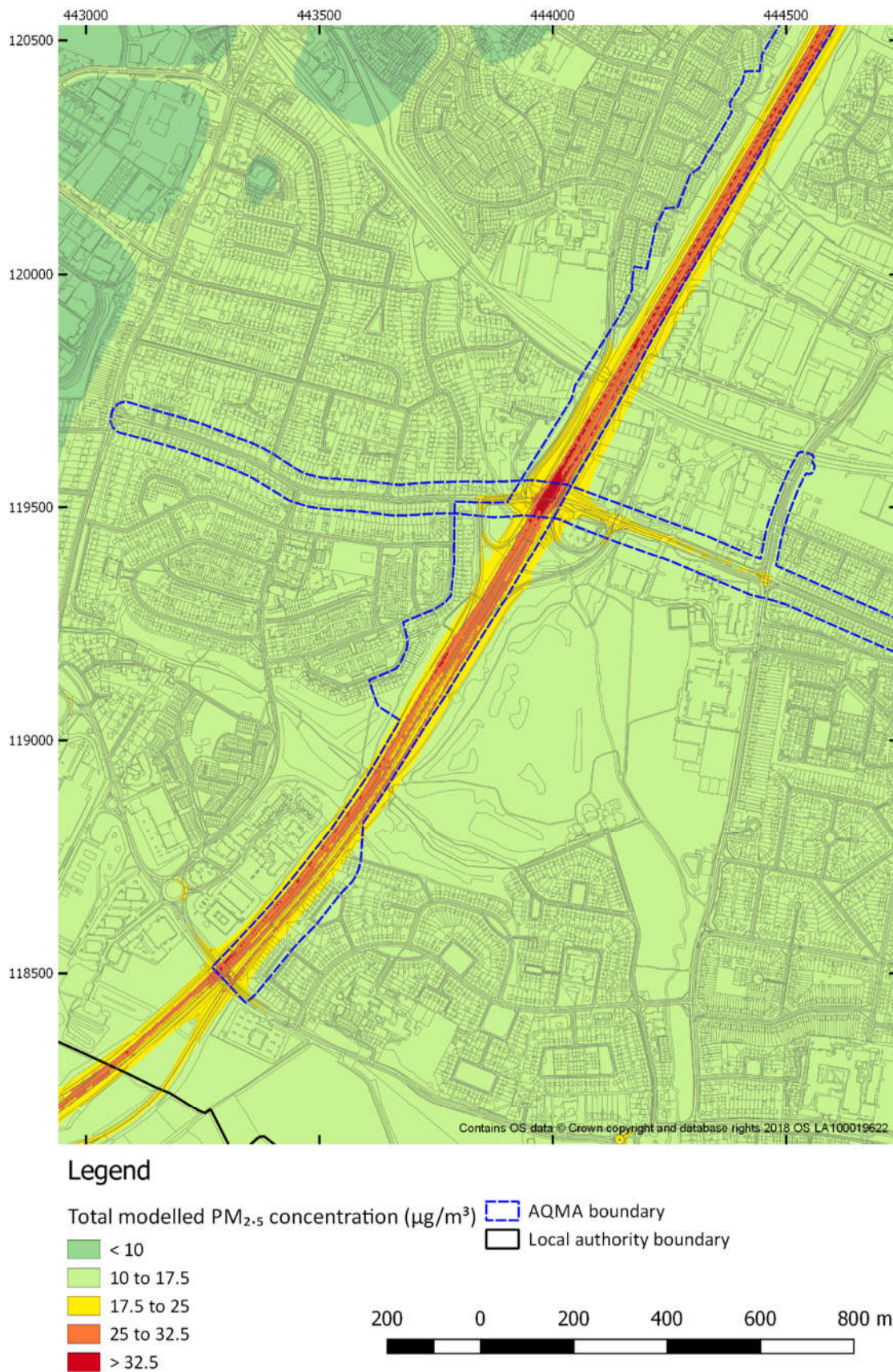
Figure 4-23 Annual mean PM 2.5 concentration model results for 2036 SGO D1 scenario AQMA No. 1 (A335 / Eastleigh) (West)
