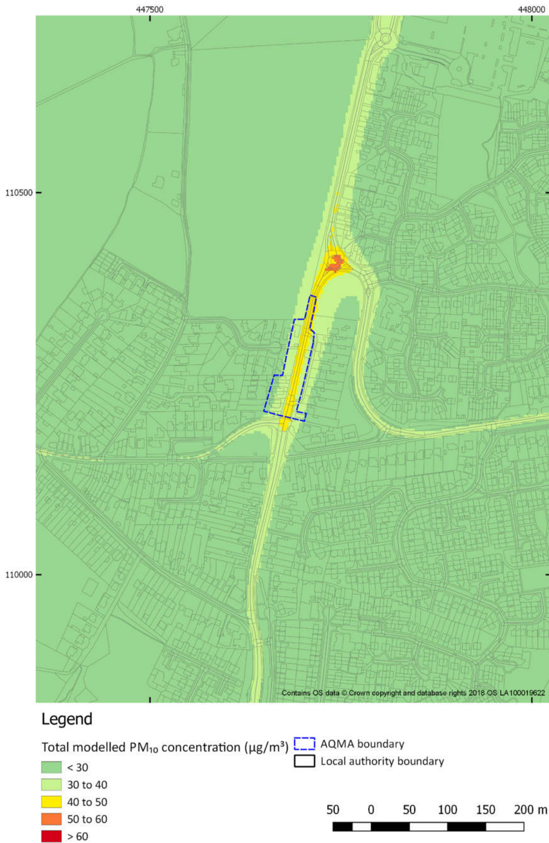
Figure 6-43 Short term PM 10 concentration model results for 2036 SGO E scenario AQMA No. 3 (Hamble Lane)
