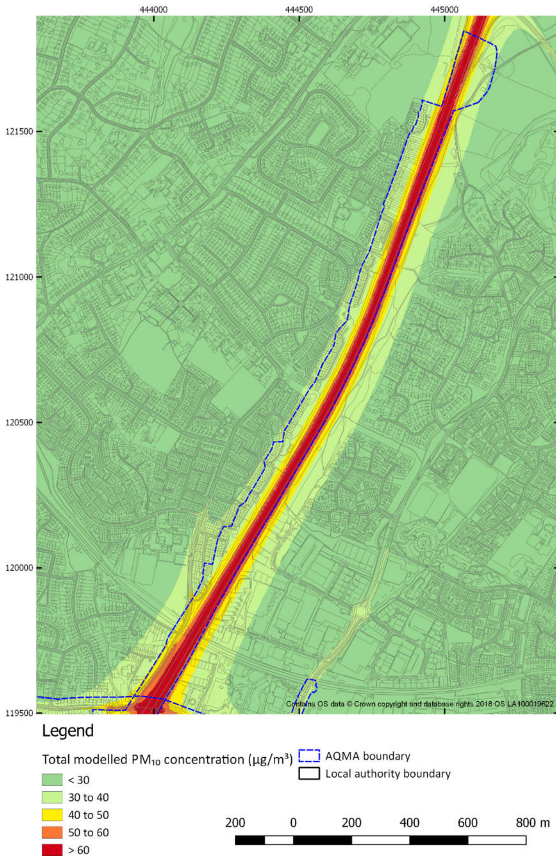
Figure 6-33 Short term PM 10 concentration model results for 2036 SGO D2 scenario AQMA No. 2 (M3) (North)
