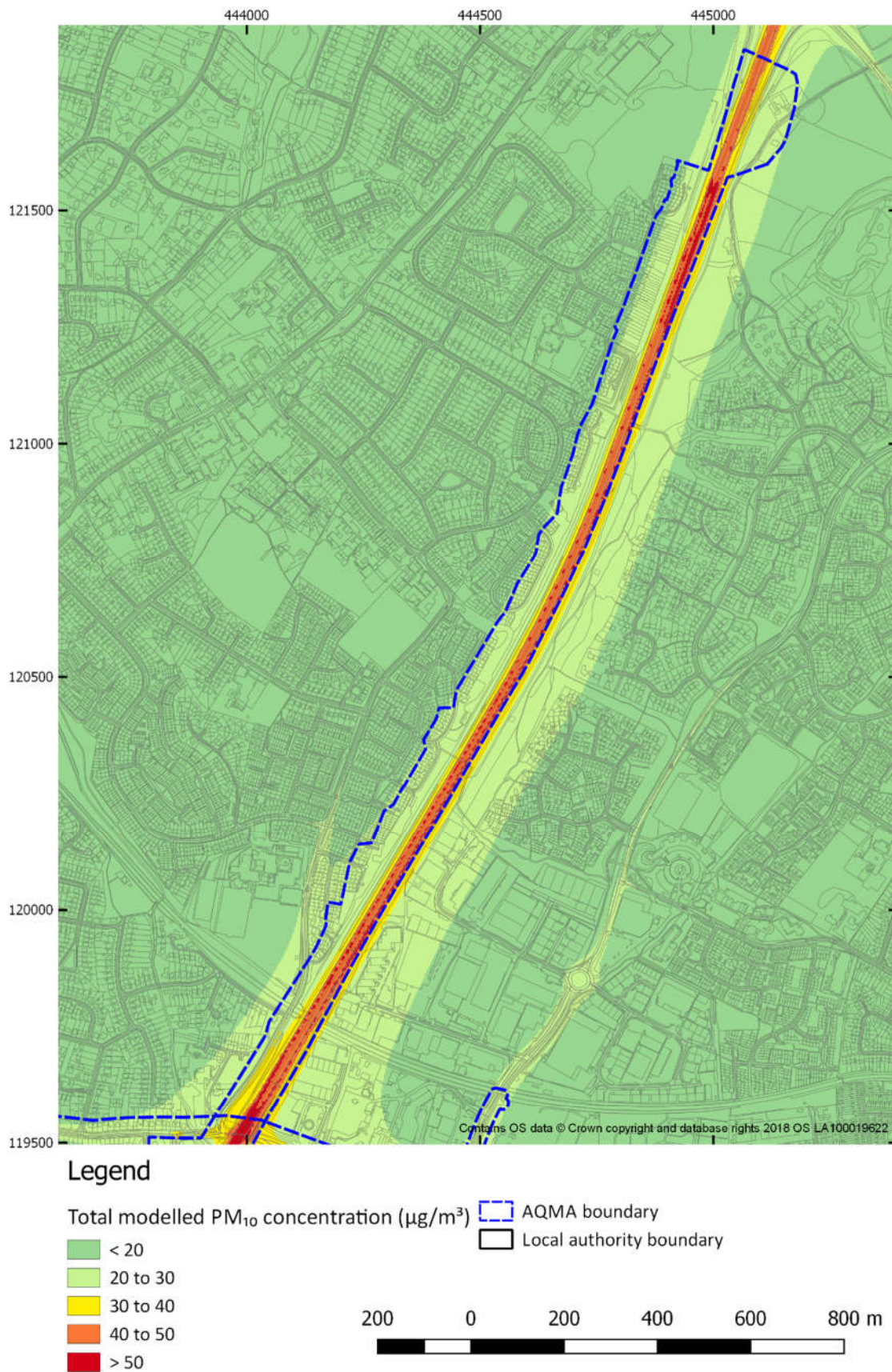
Figure 3-33 Annual mean PM 10 concentration model results for 2036 SGO D2 scenario AQMA No. 2 (M3) (North)
