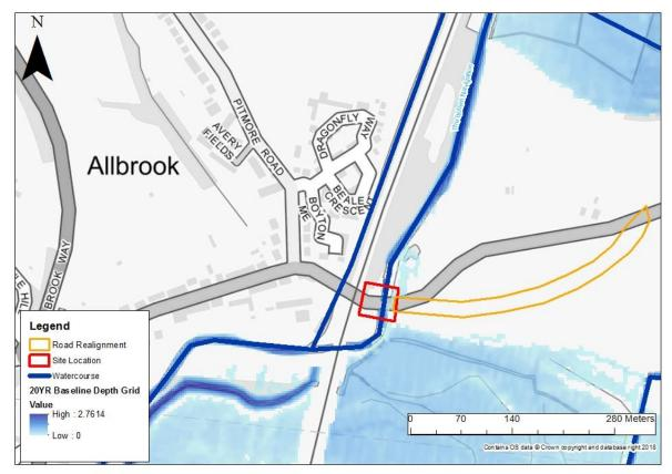
Water gets out of bank on the east bank of the Itchen Navigation directly upstream of Allbrook Hill Road bridge in the 1 in 20-year baseline scenario (Figure 5-2). A low elevation spot along the eastern bank appears to allow water to spill out onto the floodplain. Water overtops the road (as it
