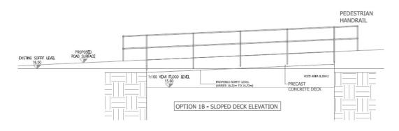
Option 1B provides optimum void space beneath the bridge, whilst also satisfying the parameters set out with regards to the road and flood levels. Moreover, the design incorporates the use of handrails instead of the existing concrete parapets provides ecological benefits to the surrounding area, facilitating the passage of light through the bridge section and minimising shading influences on the local ecology.
