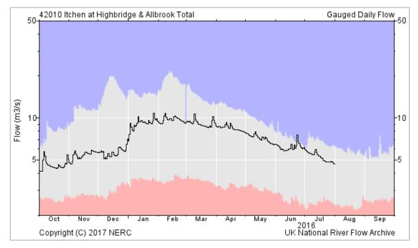
Figure 3-4: Gauged daily flow for the River Itchen at Highbridge & Allbrook
