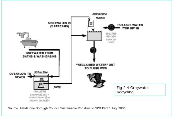
The installation of a grey water recycling system is more costeffective and less energy-intensive if incorporated at the outset of construction.
