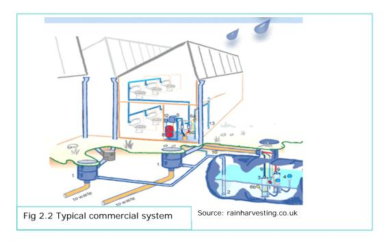
Grey water is the water that has already been used in hand basins, baths and showers. It can be recycled to save up to 49 litres per person per day(I/p/day) representing on average 33% of household water use. After basic processing, the water can be reused around the home, including flushing toilets, watering the garden or general cleaning purposes i.e. windows, floors etc
