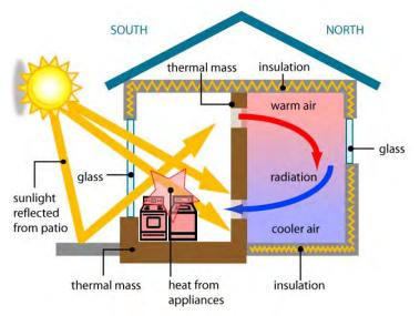
Fig 3.4 The principle of passive solar heat gain
