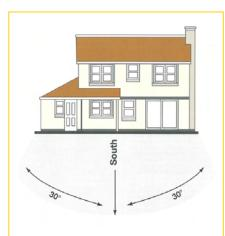
The ideal orientation for PSD is within  $30^{\circ}$  of south.
