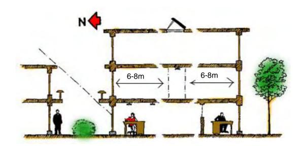
Fig 3.1 Maximum dimensions for daylight for a single aspect office
